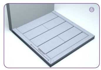
Trim the L corner at a suitable angle and fix with screw. The spacing of the screws should be no more than 500mm.
