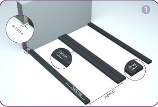
Fix the joists to the ground with expansion screws, the joist spacing should not exceed 350 mm. Double joists are needed at the end-to-end joint between decking boards.
