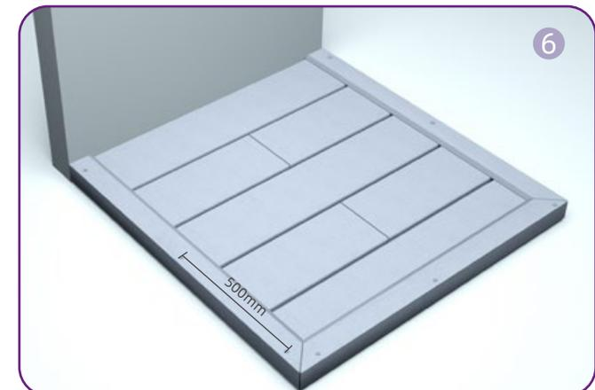
Trim the L corner at a suitable angle and fix with screw. The spacing of the screws should be no more than 500mm.
