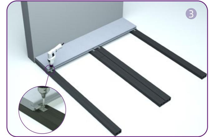
Slide the clips into the groove of the decking boards, secure the clip with screws.
