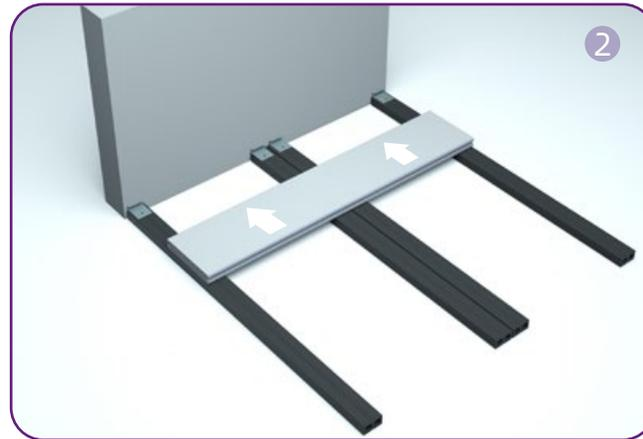
Install the start clip and slide the first decking board into the start clip.
