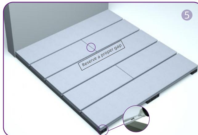
Reserve a proper gap at the butt of the two boards for contraction and expansion. Along the edge, toenail screw to secure the decking boards.
